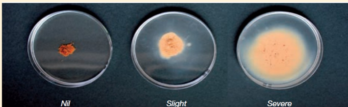
Above: Expected responses to Jar test if soil is not sodic, slightly sodic or severely sodic. Source: Department of Agriculture and Food WA, Farmnote 386 'Identifying dispersive soils
