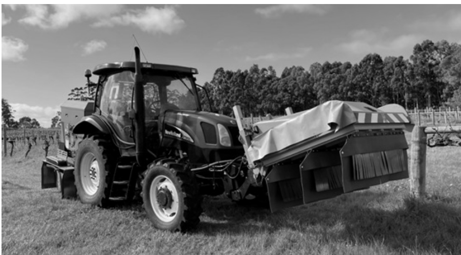
Figure 1. The AGXTEND XPower electric weed control machine, powered by Zasso™. Mounted on the rear linkage is the power unit with XPS (viculture application unit), and the XPU (urban application unit) is mounted on the front. Note that a tractor can carry either applicator, in varying configurations.
