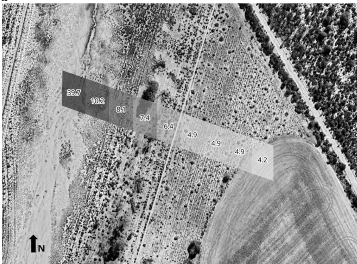
Figure 1. Transect of EM38 readings (dS/m) from the current cropping area to a saline valley floor. Readings were taken in ECa (apparent soil electrical conductivities) and were converted to ECe (soil saturation extract) by the following calculation for deep sands: ECe = 4.72ECa + 112 . The yellow line indicates where cropping may expect to show yield penalties.
